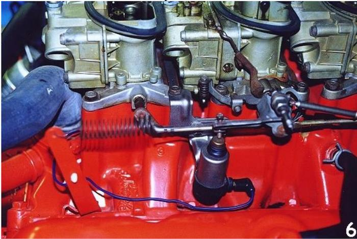
mounted to the rear of the front 2-bbl. The two rear carb (to intake) bolts secure the unique bracket, figure 6. The ID
