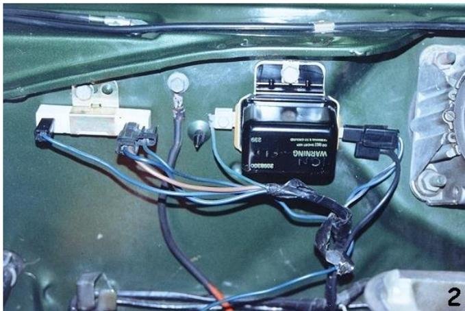
The separate "hot" wire, not part of the wiring harness, is used to activate the solenoid. This wire is a special heat resistant wire, 55 inches long and very dark brown in color. One end (a unique dual plug head, figure 2) attaches to the voltage regulator and the other to the positive terminal on the bottom of the solenoid.
