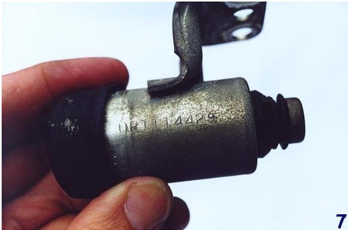
number, DR1114429, figure 7, is stamped on the side of the barrel and faces the front (radiator) of the car. The plunger (adjustable) should have a brass ROUND head. The solenoid wire, medium blue in color, is incorporated in the wiring harness. The throttle return spring bracket incorporates a special nylon clip (usually white or black) that holds the wire.
