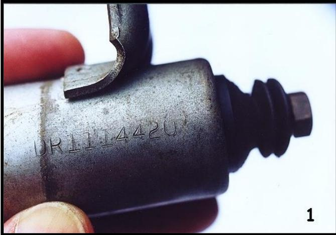
All 69 1/2 440-6 engines used the same solenoid mounted to the left side of the intake manifold. The solenoid plunger (which is adjustable) should have a brass HEX head. All solenoids are stamped with an identification number that faces the front (radiator) of the car. The 69 1/2 I.D. number is DR1114420 (see figure 1.) This is the ONLY number research has shown to be used on these cars.
