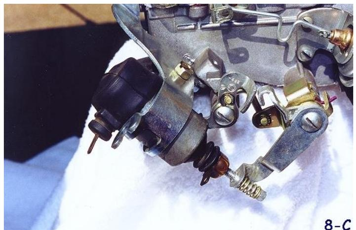
All 1970 440-6 engines used the same solenoid mounted to the left side of the intake manifold. The solenoid plunger (adjustable) should have a ROUND brass head. The ID number, DR1114429, (same as fig. 7) is stamped into the barrel of the solenoid and faces the front (radiator) of the car. The positive wire, medium blue in color, connects to the terminal at the bottom of the solenoid. The wire is a part of
