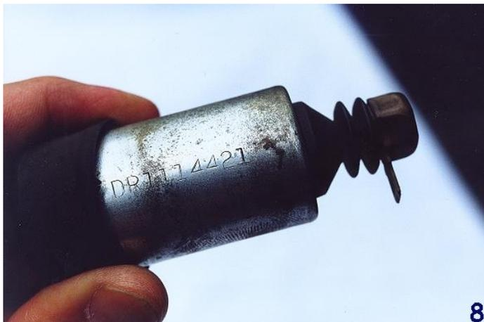
All AVS equipped 440-4bbl. engines utilized a solenoid mounted in a special bracket attached to the right side of the carb. The bracket is the same as used on the 340-4bbl. AVS, the solenoid however, is quite different. The ID numbers found for this application are (generally found on 70 cars) DR1114421 and (generally found on 71 cars) DR1114447 (figures 8 and 8A respectively) stamped into the side of the
