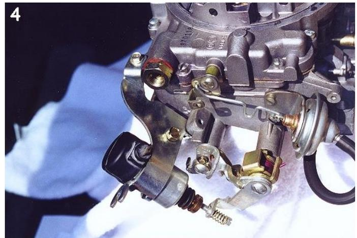
bracket used. However the ID numbers found for the application are DR1114442, figure 5. The plunger (which is adjustable) should have a brass ROUND head. There is one positive (hot) wire connected to the terminal at the bottom of the solenoid.
