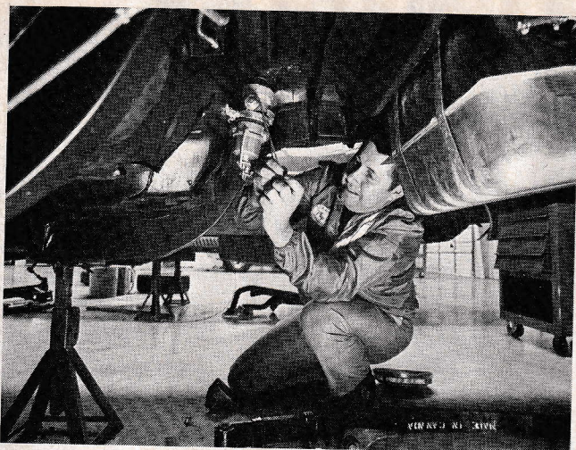
Stewart Warner fuel pump was mounted at rear near gas tank to insure maximum fuel supply. Hey, Ronnie & Buddy, what's that funny spring with the 'Made in Canada' sign doing on your match racer?
