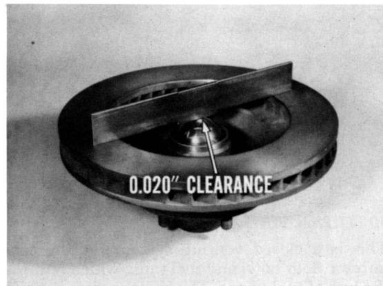
Fig. 32—Inner surface removal gauging
