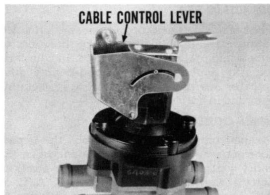
Fig. 18—Barracuda and Challenger water valve
