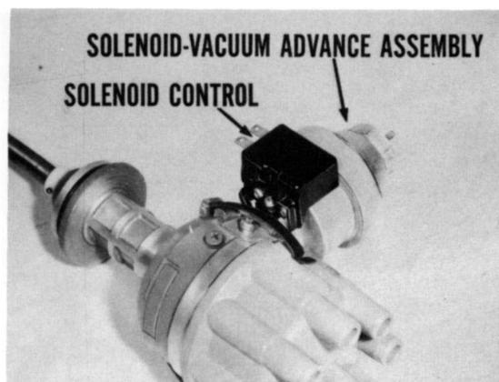
Fig. 27—Solenoid retards timing at idle
