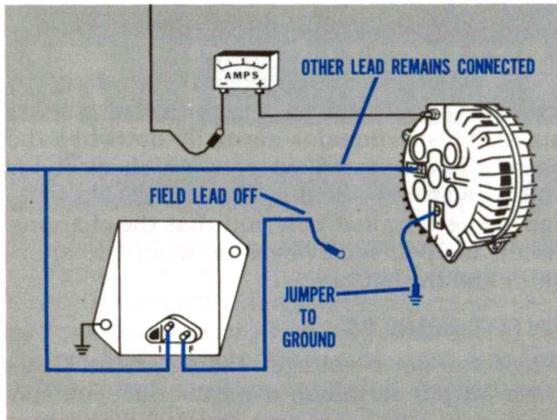
Fig. 23—Charging Circuit Resistance Test connections
