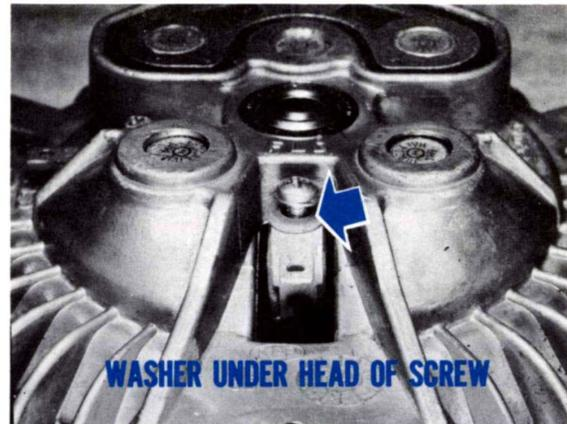
Fig. 34—Make sure washer is in place
