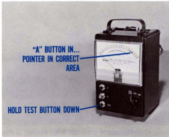
Fig. 14—Regulator Test—2nd Step
