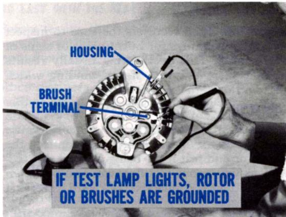
Fig. 32—Internal Field Circuit Ground Test
