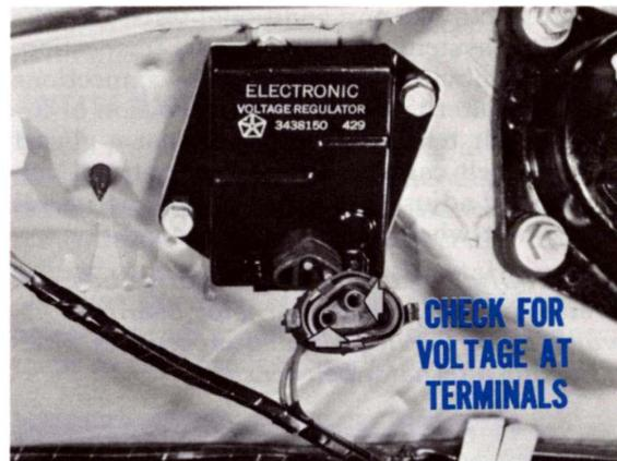
Fig. 16—Check voltage with tester prod
