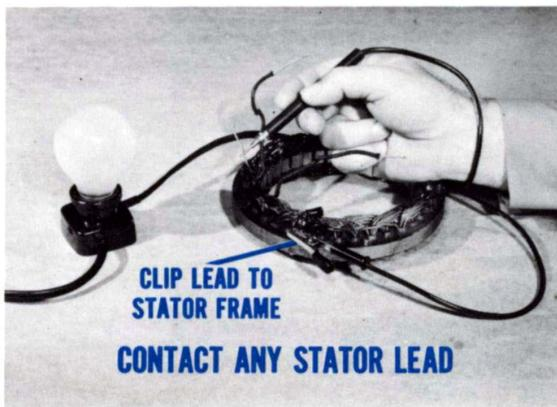
Fig. 39—Stator Ground Test
