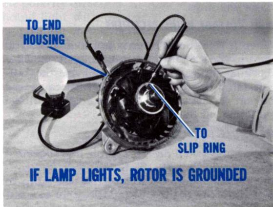
Fig. 33—Rotor Ground Test
