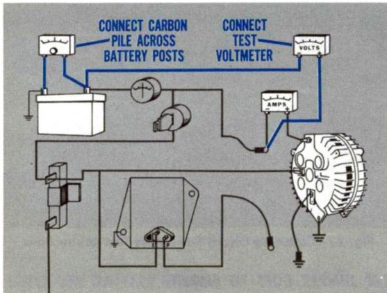
Fig. 24—Voltmeter and Load connections
