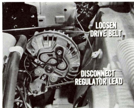
Fig. 19—Prepare for Current-Draw Test
