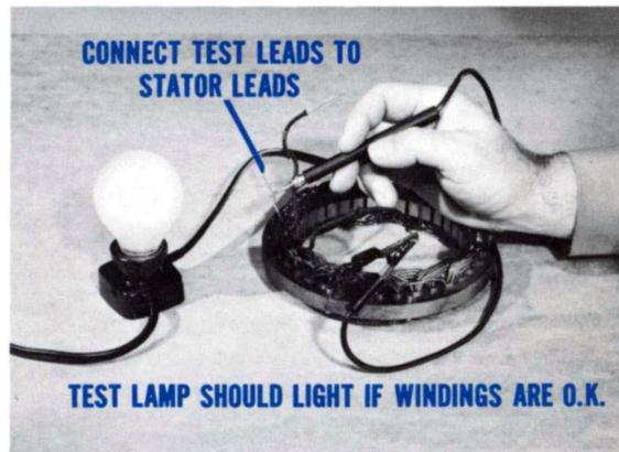
Fig. 40—Stator Continuity Test
