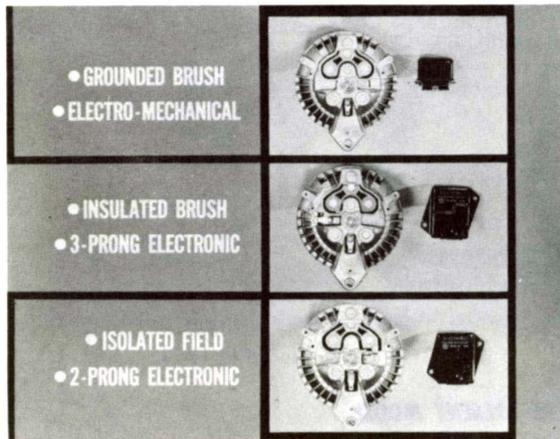
Fig. 4—Alternator and regulator must match
