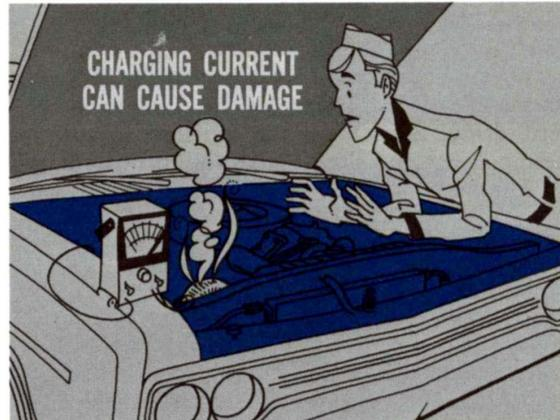
Fig. 25—Keep engine speed low
