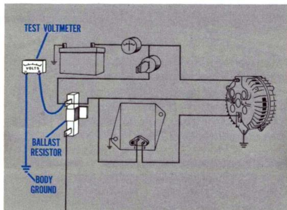
Fig. 30—Charging Voltage Test connections
