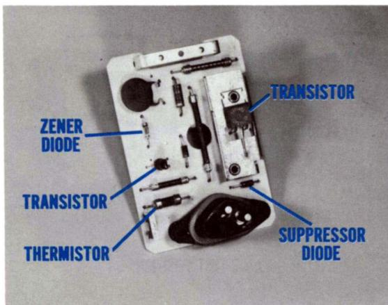
Fig. 8—Electronic regulator components
