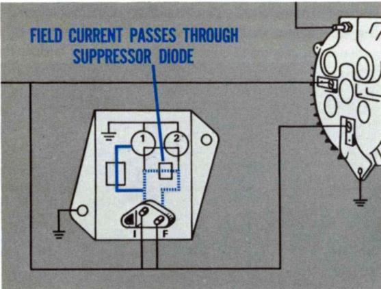
Fig. 11—Suppressor diode reduces field current
