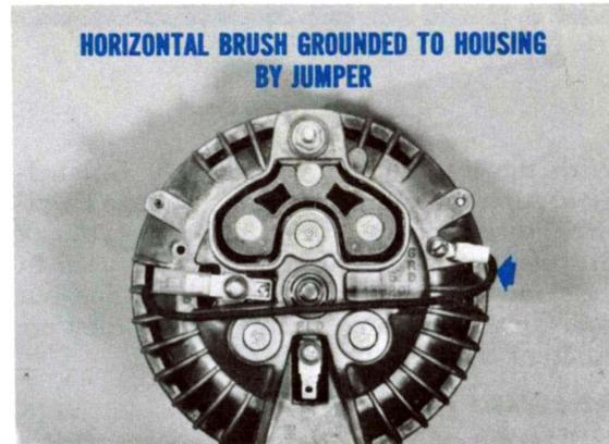
Fig. 5—Modification for light-duty trucks
