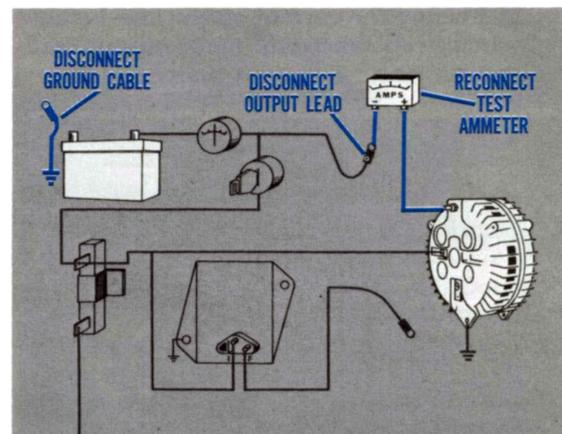
Fig. 22—Charging Circuit Resistance Test connections
