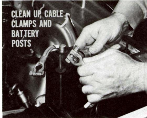
Fig. 18—Eliminate possibility of resistance
