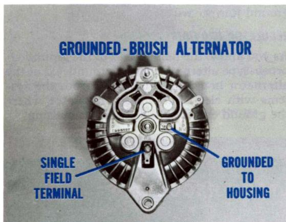
Fig. 1—Used with electro-mechanical regulator
