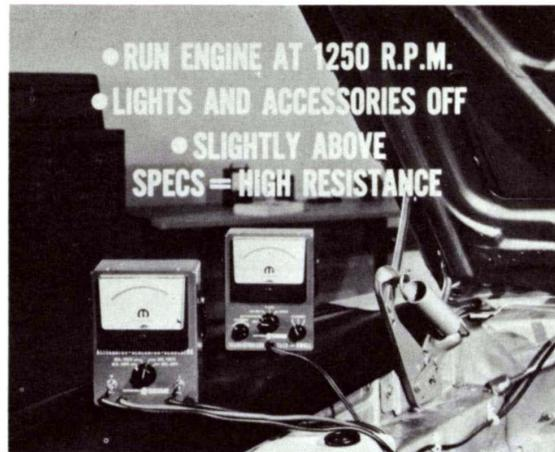
Fig. 31—Charging Voltage Test
