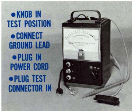
Fig. 12—Voltage regulator tester connections
