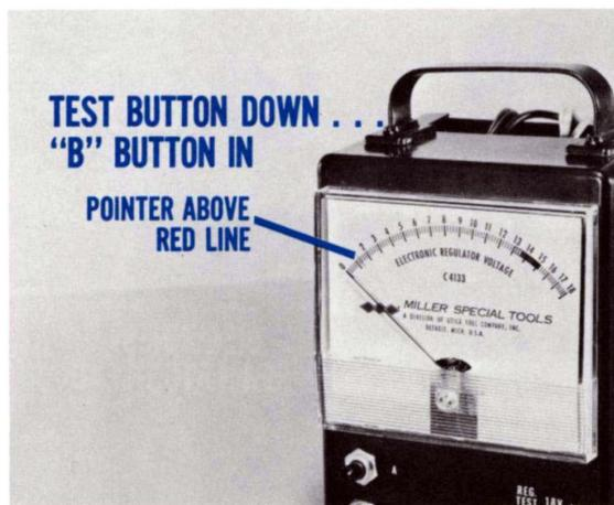
Fig. 15—Regulator Test—3rd Step
