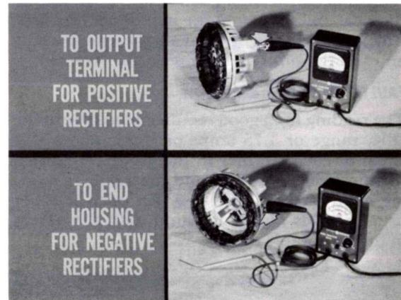
Fig. 35—Rectifier Tester connections
