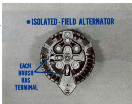
Fig. 3—Used on all 1970 Chrysler-built cars
