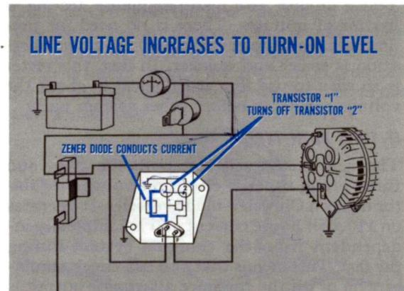
Fig. 10—Voltage "triggers" Zener diode
