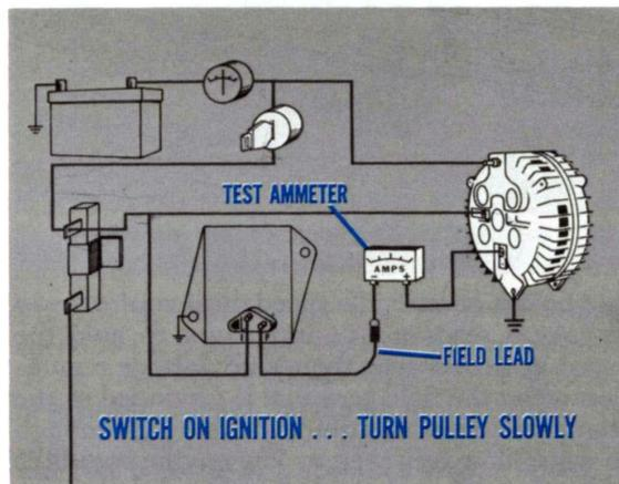
Fig. 20—Current-Draw Test conditions
