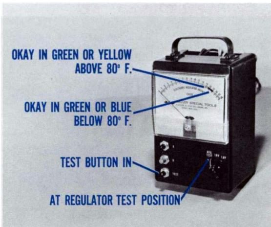
Fig. 13—Regulator Test—1st Step
