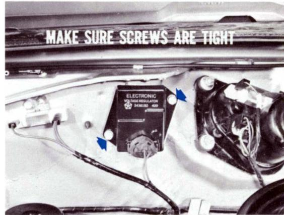
Fig. 28—Regulator must have a good ground
