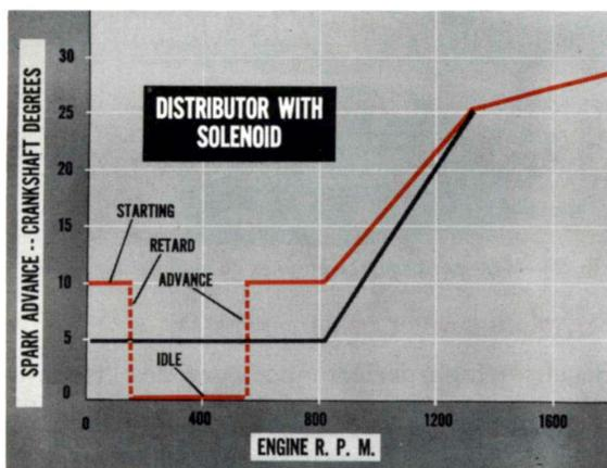
Fig. 17—Ignition advance curve comparison
