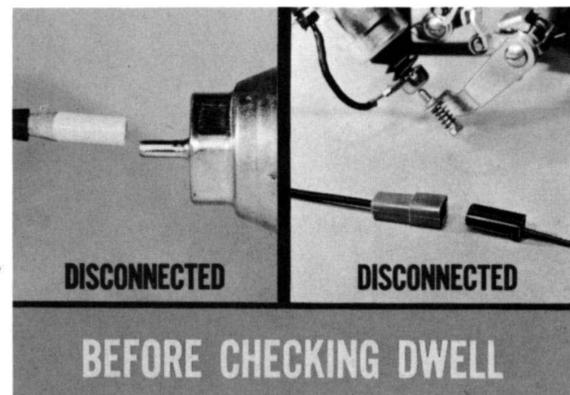
Fig. 35—Disconnect both the solenoid and the vacuum
