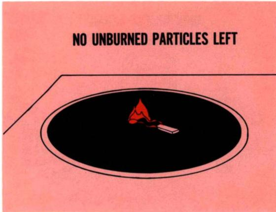
Fig. 9—Closely packed particles burn completely
