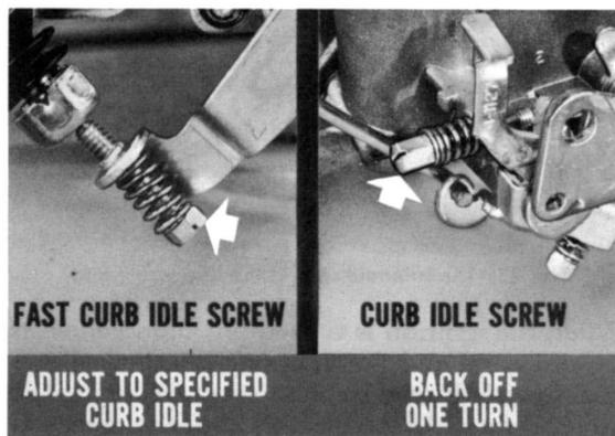
Fig. 27—Adjust both of the curb idle screws
