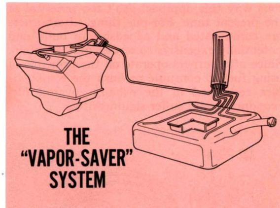
Fig. 2—Fuel vapors are vented to the engine crankcase
