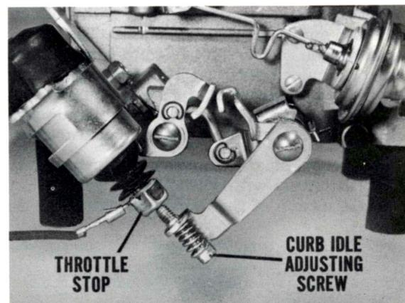
Fig. 19—Carburetor controls the distributor solenoid
