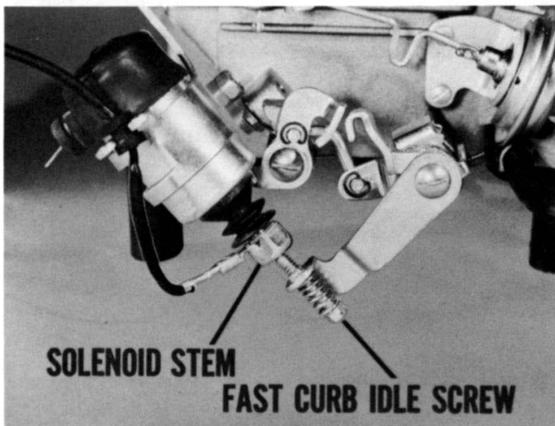
Fig. 23—The solenoid stem is the idle screw stop
