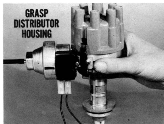
Fig. 30—Don't use the vacuum unit as a turning handle
