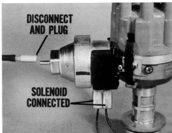
Fig. 29—Do not disconnect the distributor solenoid
