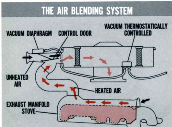
Fig. 16—A heated air blending system is used
