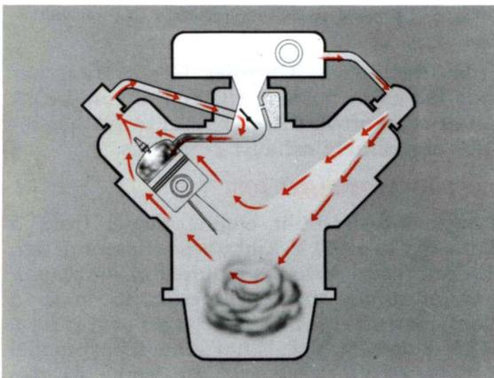
Fig. 1—The closed crankcase ventilation system
