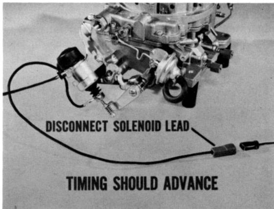
Fig. 31—To check distributor solenoid operation
