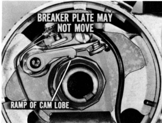
Fig. 33—This is not a valid solenoid test
