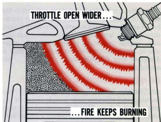
Fig. 12—More mixture for more complete combustion
