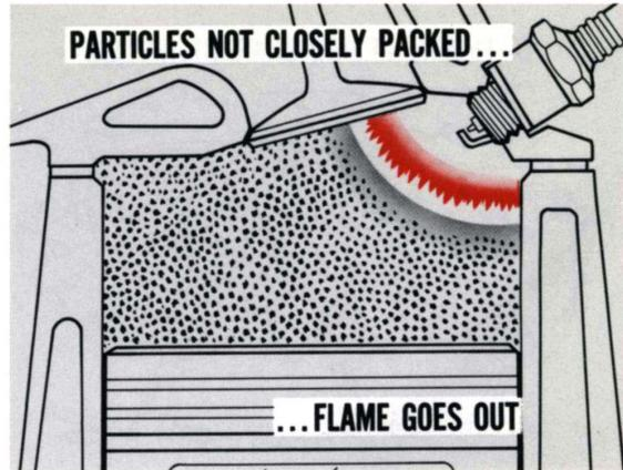
Fig. 11—Not enough mixture to support combustion
