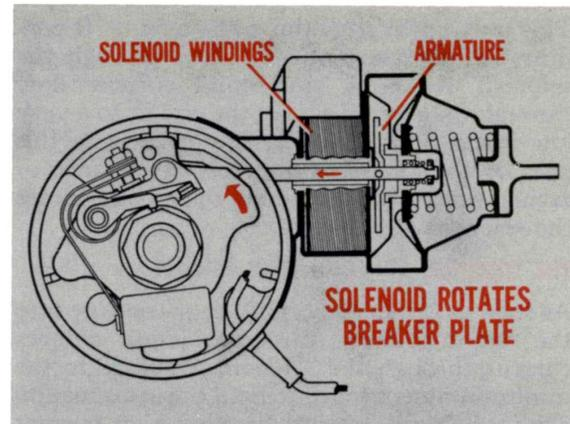
Fig. 18—The solenoid is built into the vacuum unit
