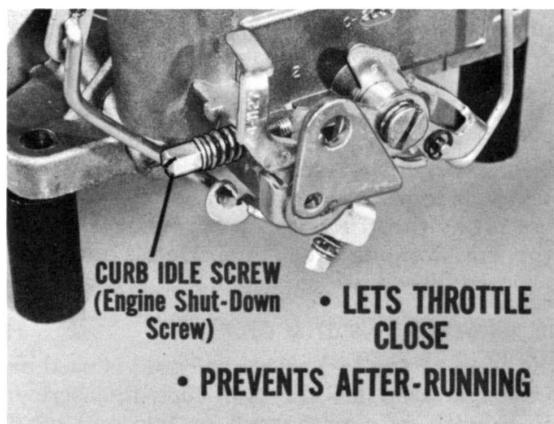
Fig. 26—It's really the engine shutdown screw
