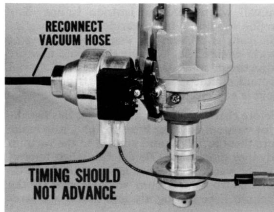
Fig. 32—If timing advances, readjust the carburetor
