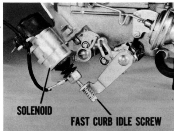
Fig. 25—They added a solenoid and changed a name
