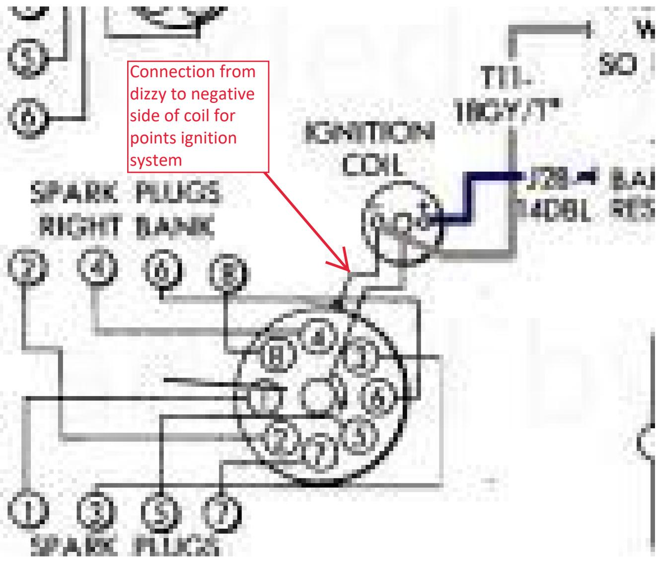
Connection from dizzy to negative side of coil for points ignition system
