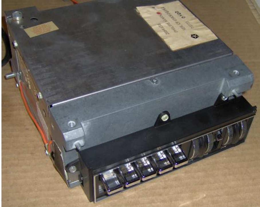
This is the bottom side of a 1970 Phillips AM FM # 2884658 . Notice the Antenna port is located on the bottom of the radio . This holds true for ALL E body radios 1970-1974 . Also note the unique location of the mounting bolt holes at the bottom front of the radio .
