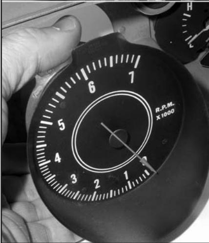
**3. Now you can remove the three nuts (around the perimeter) that retain the tach and pull it out. Don't remove any of the other nuts at this time.**
