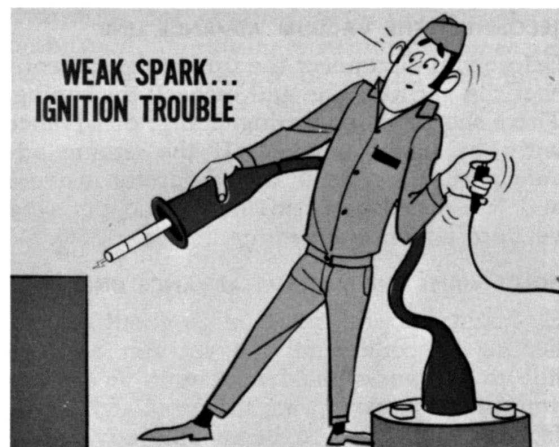
Fig. 18—If spark is weak, check primary circuit resistance
