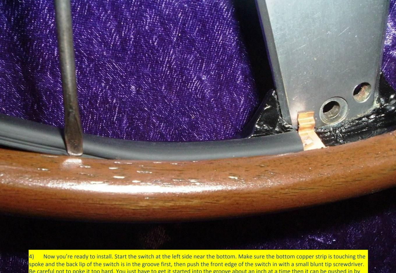
Be careful not to poke it too hard. You just have to get it started into the groove about an inch at a time then it can be pushed in by hand. Repeat this one inch procedure all the way around. WWW.RIM-BLOW.COM
