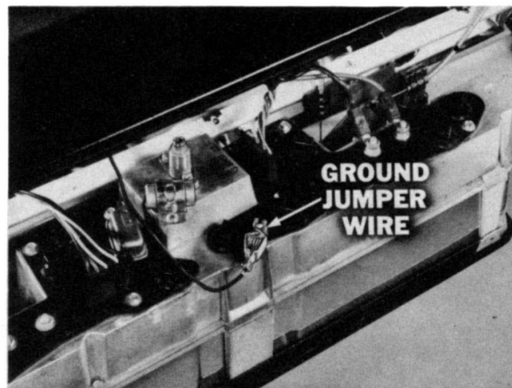
Fig. 19—Ground jumper protects gauges
